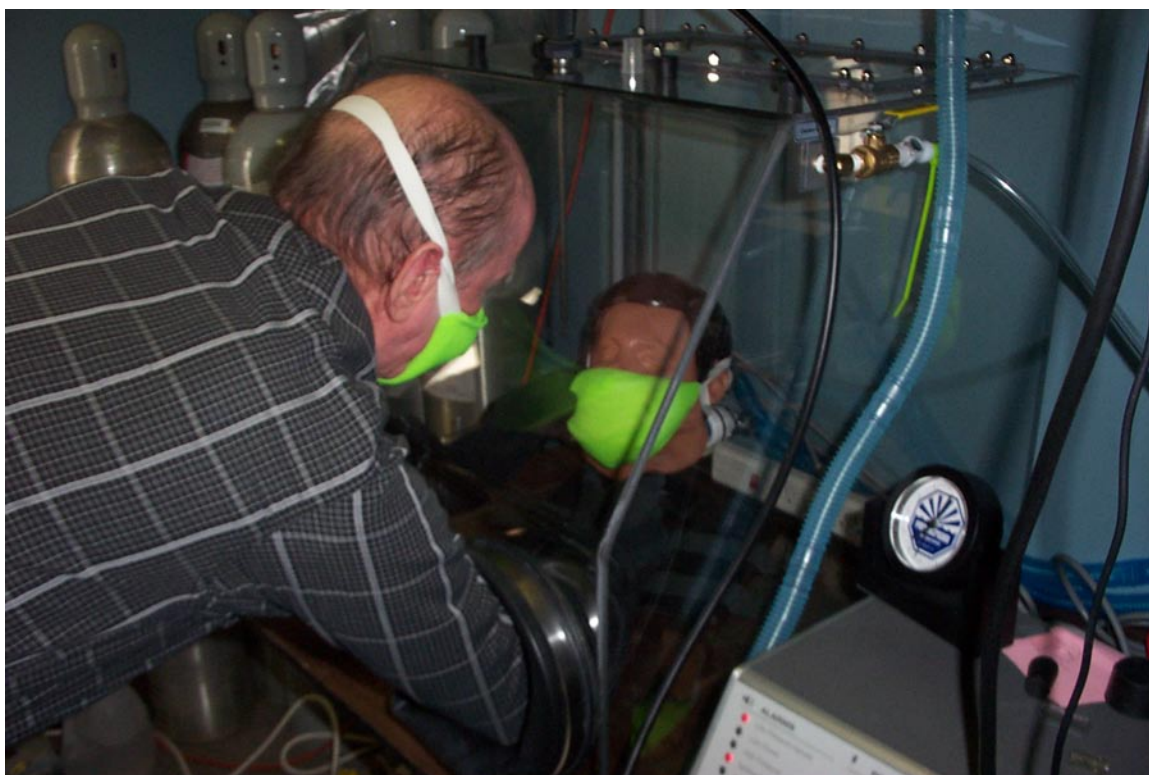
Figure 5. Massaging a Smoke Mask During Active Test
