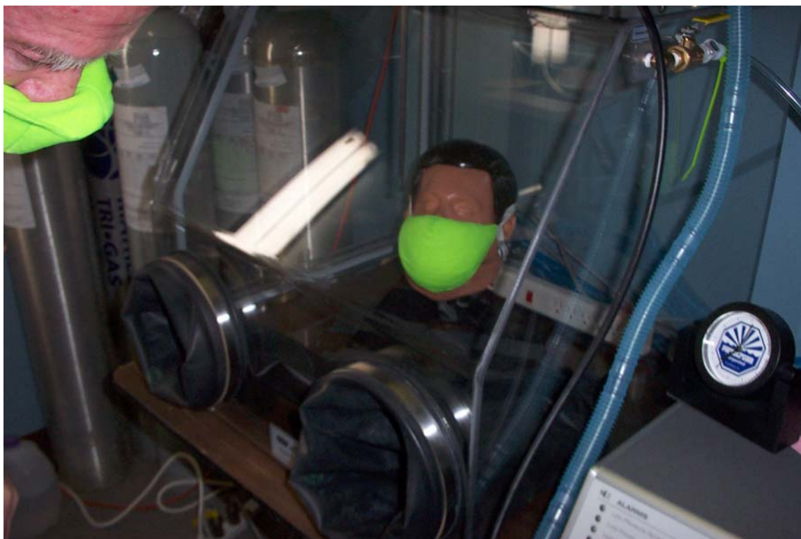
Figure 2. Mask Mounted on Human Head Simulator Inside Plexiglas Glove Box
