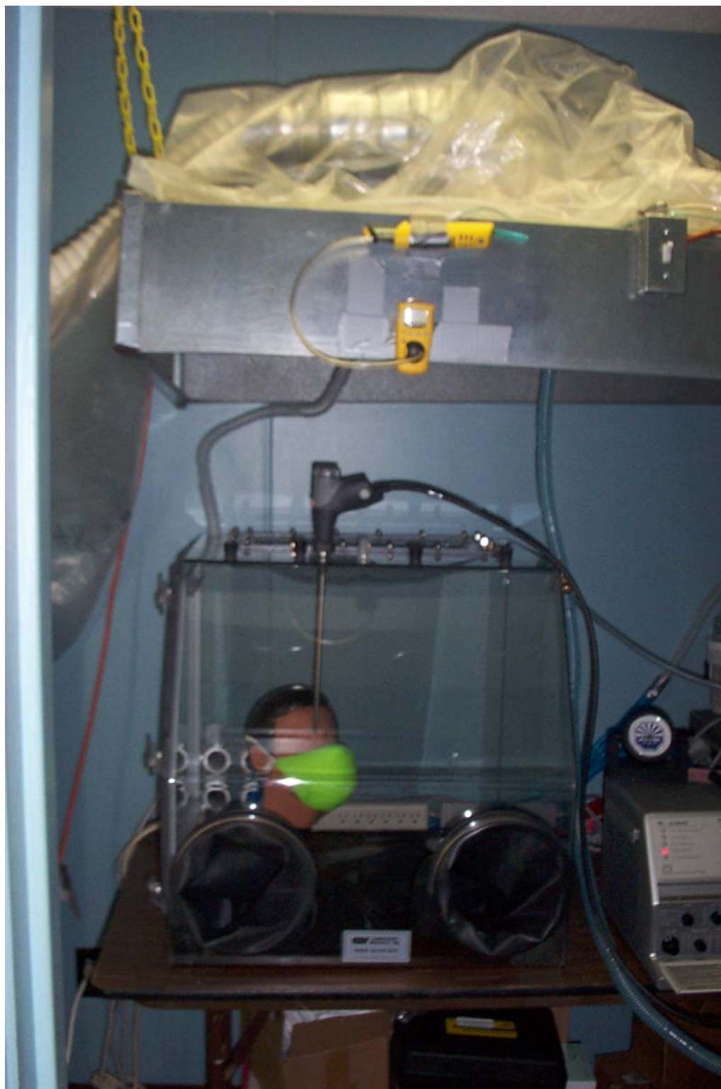
Figure B. Filter Mask For Testing Mounted On Human Head Simulator In Glove Box
